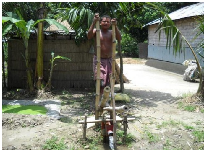
Running costs are close to zero but treadle pumps are labor intensive.
