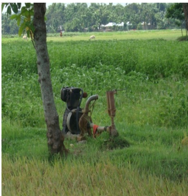
An old treadle pump has been recycled for priming a diesel engine.
