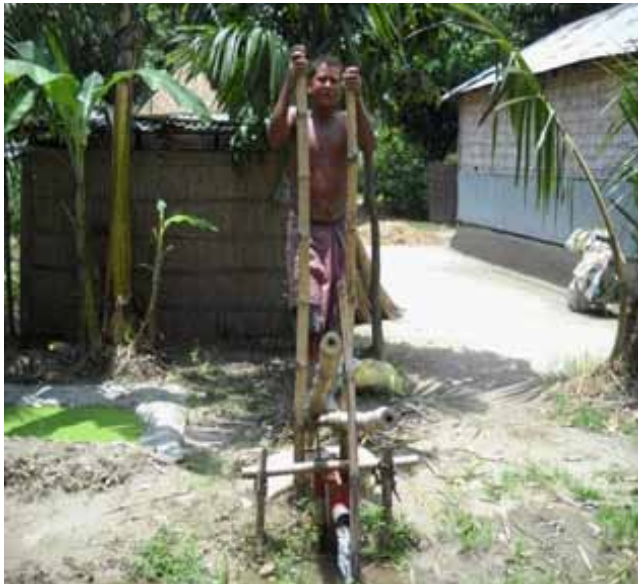
Farmer using a treadle pump
