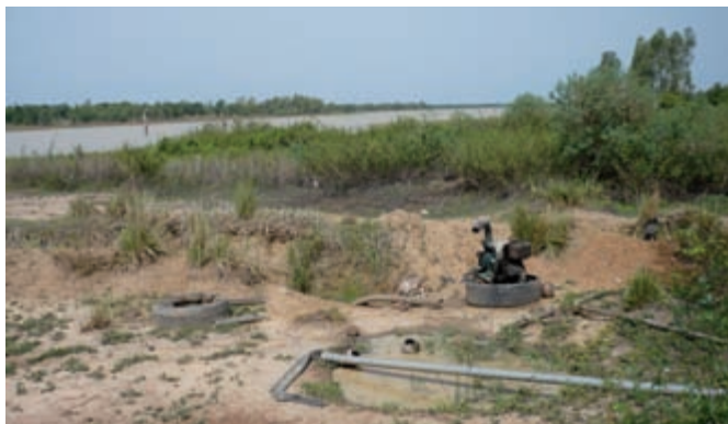
Figure 5: Motorpump withdrawing from hand dug dike for irrigation on shores of small reservoir
